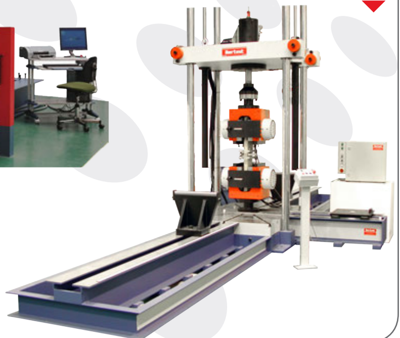
▶ Ensayos de grandes elementos de madera Testing on large timber elements
