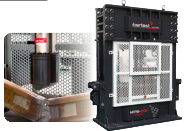
▲ Rotura a flexión estática de carriles Static flexure testing for railway tracks
