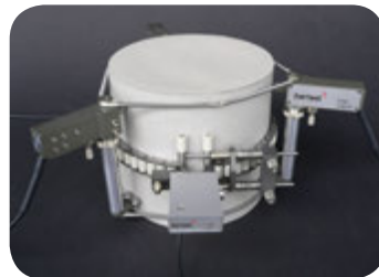
▶ Elasticidad de rocas y hormigones Rock and concrete compression elasticity
